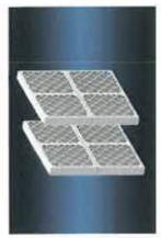
First filtration stage: Disposable panel filters • Halton pleated filter G4 (EU4) • Purpose: remove large particulate • Efficiency > 95% (efficient for 5 microns and above) Replacement frequency assumes high efficient KSA cyclonic filters are used in the hoods or in the ventilated coilings as primary filters. Regular replacement helps to support the longevity of the disposable bag filter.
